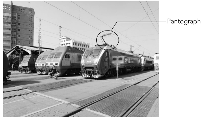
Figure 1.7 OCS and Electric Locomotives
