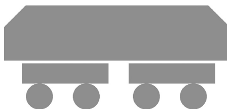
Figure 1-3 B_0-B_0 wheel arrangements
